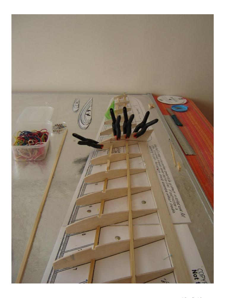
Upper front spar still not glued btw, only the main wing upper rear spar which acts as lower rear spar for the wing tips.
